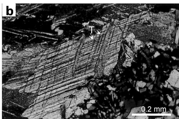
Fig. 10 Photomicrographs of calcite twinned twins (1) (mechanical e-twinning of calcite, dark lines indicated by arrows labeled T). (a) Twinned twins in the sample Ta-2 showing the twin density 63/mm. (b) Twinned twins in the sample Ta-3 showing the twin density 77/mm. Upper (Crossed nicols), lower (Crossed nicols).
